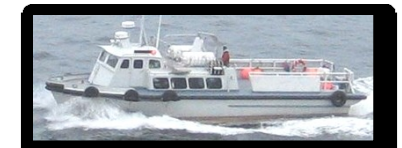
Crew/Utility Boat – Cape Lookout 40 Passengers/2 Crew Length: 48 Ft - Width: 17Ft - Depth: 7 Ft Horsepower: 1320
