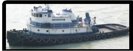
Tug – Le Cheval Rouge Length: 91 Ft - Width: 30 Ft - Depth: 13 Ft Horsepower: 3,400
