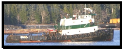
Tug - Muzon Length: 86 Ft - Width: 26 Ft - Depth: 12 Ft Horsepower: 2,000
