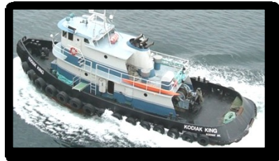
Tug – Kodiak King Length: 71 Ft - Width: 25 Ft - Depth: 8 Ft Horsepower: 3,000
