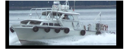
Crew/Utility Boat – Vallendar 20 Passengers/2 Crew Length: 42 Ft - Width: 15 Ft - Depth: 7 Ft Horsepower: 1006
