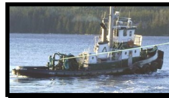
Tug – Cape Arago Length: 62 Ft - Width: 17 Ft - Depth: 8 Ft Horsepower: 1,275
