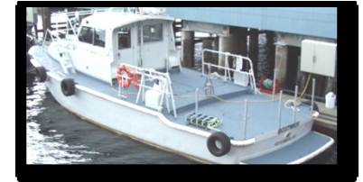
Crew/Utility Boat – Bostwick Length: 41 Ft - Width: 14 Ft - Depth: 4 Ft Horsepower: 1,006
