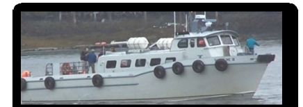
Crew/Utility Boat – Shoreline IX 49 Passengers/2 Crew Length: 62 Ft - Width: 17 Ft - Depth: 7 Ft Horsepower: 960
