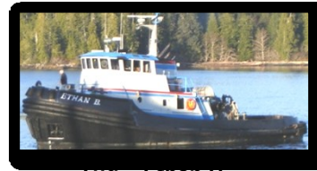
Tug – Ethan B Length: 63 Ft - Width: 26 Ft - Depth: 11 Ft Horsepower: 2,200
