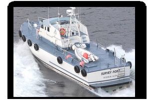
Crew/Utility Boat – Survey Point Length: 66 Ft - Width: 18 Ft - Depth: 9 Ft Horsepower: 2200
