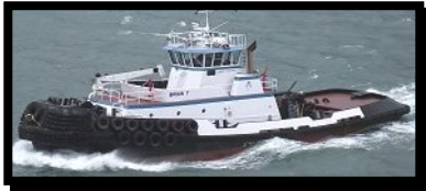
Tractor Tug - Brian T Length: 117 Ft - Width: 36 Ft - Depth: 15 Ft Fire Fighting Equipped Horsepower: 4,400
