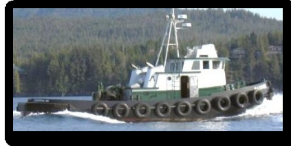
Tug – Banner Length: 51 Ft - Width: 19 Ft - Depth: 9 Ft Horsepower: 900
