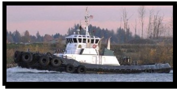
Tractor Tug – Anna T Length: 105 Ft - Width: 36 Ft - Depth: 17 Ft Fire Fighting Equipped Horsepower: 4,400
